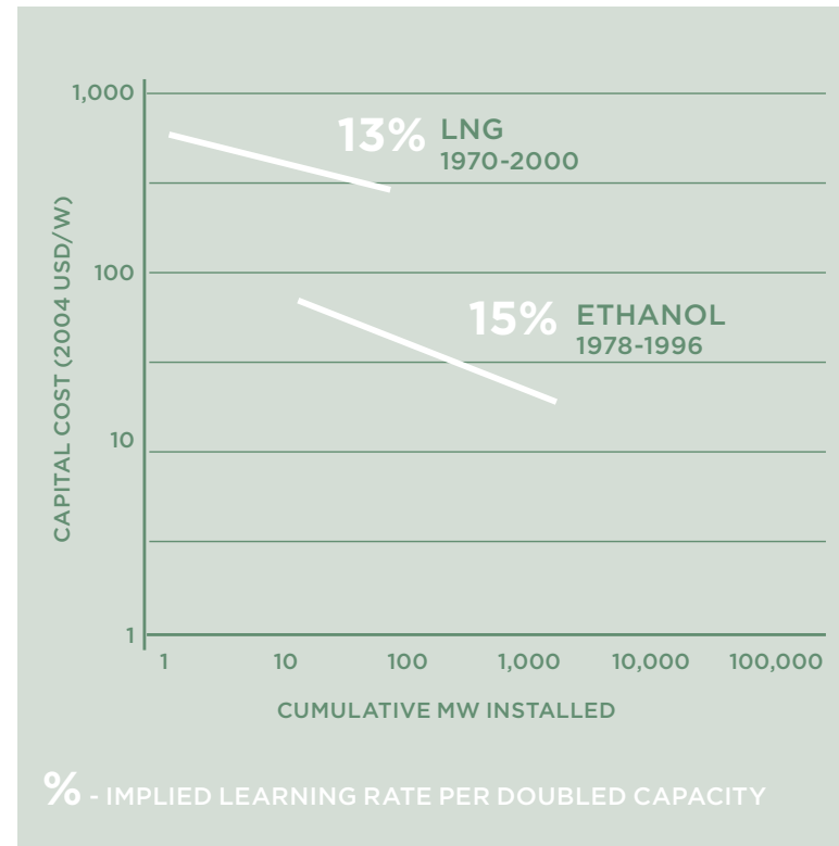
▲ 'Learning by Doing' for energy industries as an analogue for CC(U)S cost reduction Based on original source: Advanced Resources International
