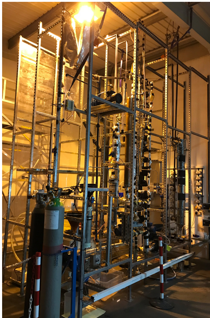
◀ Pilot testing apparatus of novel c-capture solvent. Image courtesy of C-Capture Ltd.
