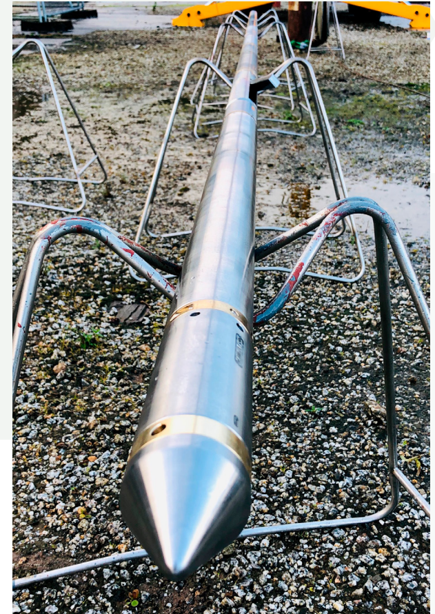
BOREHOLE MICROGRAVITY TOOL. IMAGE COURTESY OF SILICON MICROGRAVITY
