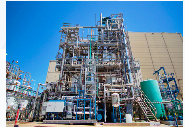
PILOT-SCALE TESTING SITE OF THE PZ SOLVENT AT THE UNIVERSITY OF TEXAS, AUSTIN. IMAGE COURTESY OF UT
