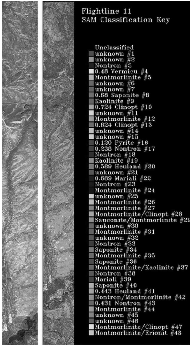
Figure 16: Detailed habitat mapping that results from an ENVI “hourglass” process. This process ended with a Spectral Angle Mapper (SAM) analysis of flightline 11 that is shown in the center. On the left is a “true color” RGB image of flightline 11.
