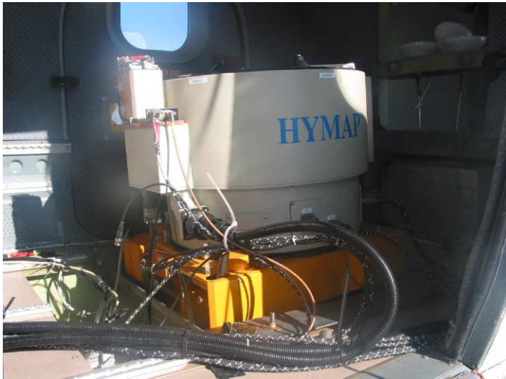
Figure 8: The hyperspectral sensor is shown in the aircraft used by our acquisition contractor for image acquisitions.
