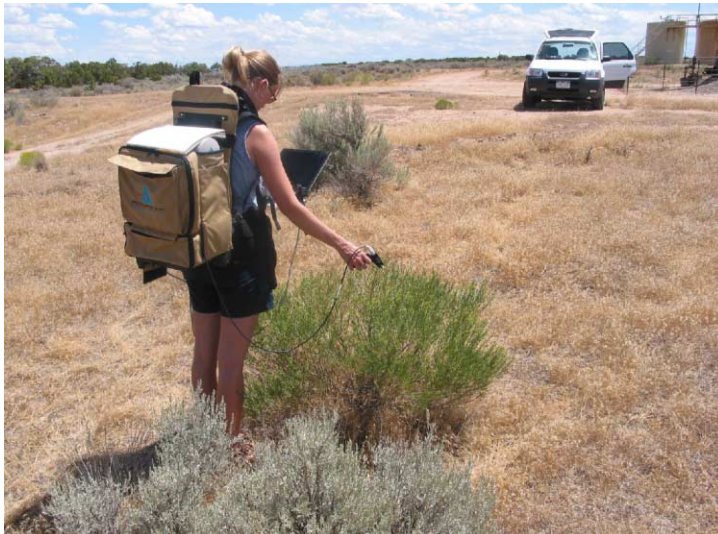
Figure 22: Measuring reflectance spectra of a plant at the border between two habitats. Notice the well pad.
