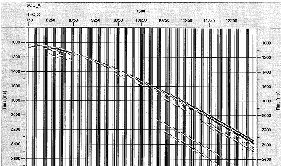
Figure 19: Change in pressure response (shot gather) between 2020 and 2005. Note amplitude change and AVO effects associated with S_w and S_{CO_2} changes in the reservoir.
