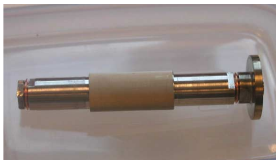
Figure 4: Photograph of a tubular module with the external protective wire mesh installed.
