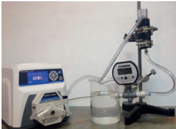
Figure 8. Apparatus for performing biomineralization sealing of shale cores and simultaneously measuring core permeability.
