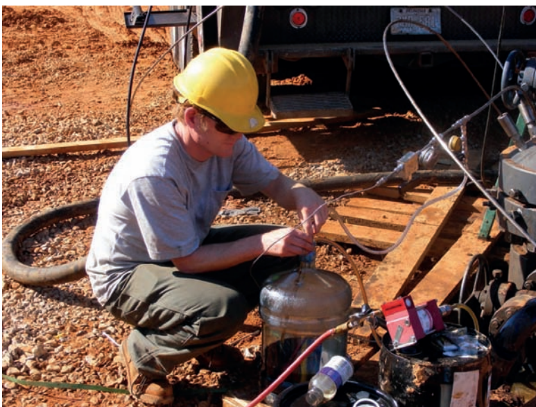
Figure 9. Setting of the hydraulic system using a small air driven piston pump. Hydraulic oil is injected down the 1/4" center tube in the tube-in-tube and returns up the outer 3/8" tube.
