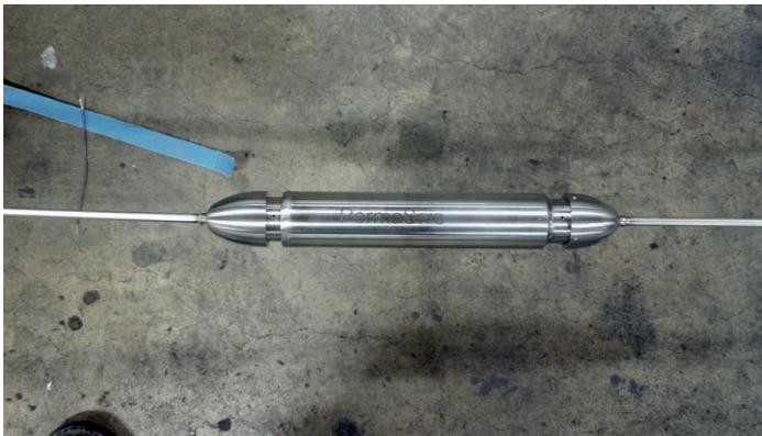
Figure 9. Geophone Pod with TEC cable attached via orbital welding.
