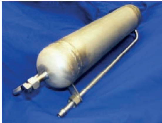
Figure 5. Pall's small scale membrane separation module (12 tube, 25.4 cm active membrane length).
