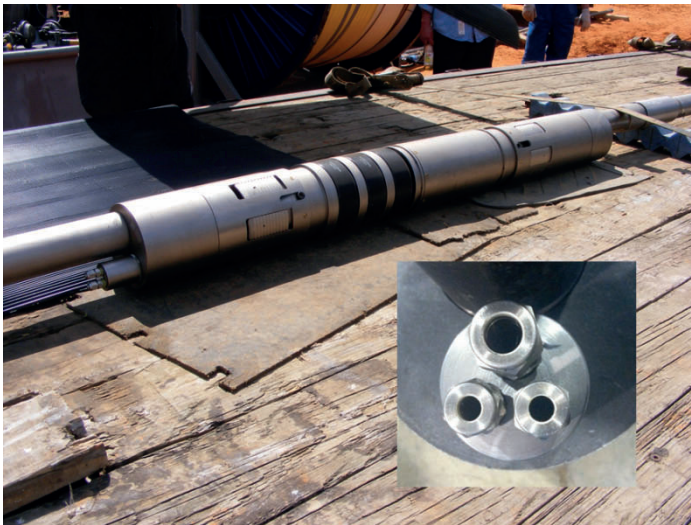
Figure 7. The D&L Hydroset II hydraulic set packer. The inset photograph shows the pass-throughs for the fiber-optic, pressure/temperature, and U-tube control lines.
