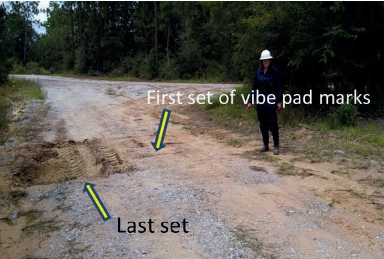
Figure 22. Effects of vibroseis sweeps at SP 2021. Multiple sets of sweeps were recorded together with the first and last set ‘pad marks’ labeled with yellow arrows. Each pad mark had 20 or 24 sweeps.
