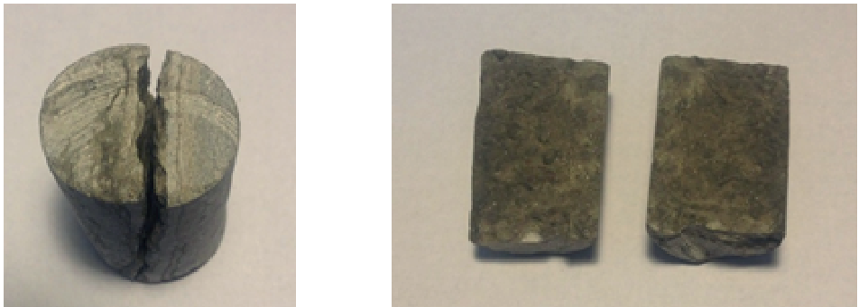
Figure 6. Split OP2-4 Core. Core length was 4.01 cm (1.58 inches).
