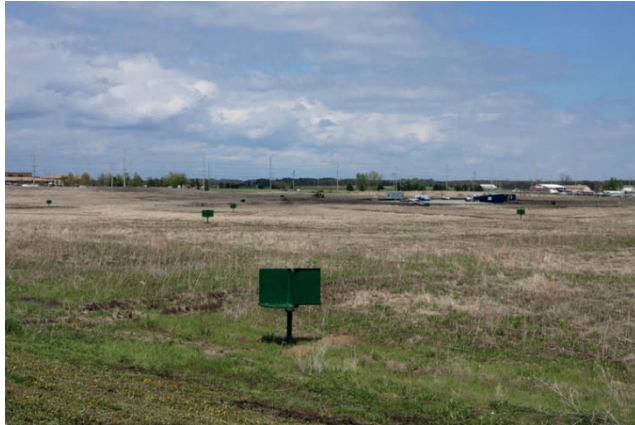
Figure 3. Artificial reflectors installed at the Decatur site.
