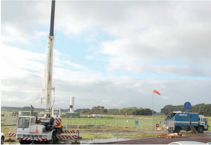
Figure 2. Logging of the Otway Project CRC-1 injection well with RST in July 2011.
