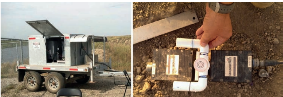
Figure 4. Left: Zonge Generator. Right: Emplacement of two sensors relative to a survey marker.
