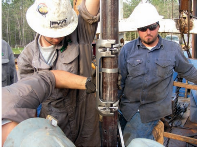
Figure 3. Installing a GCDT Inc. control line protector over the fiber-optic cable termination to protect it while running-in-hole.
