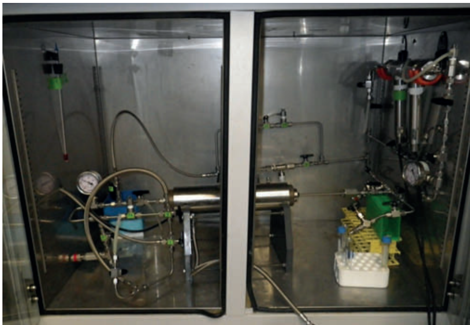
Figure 12. The high pressure core test system. The Hassler type core holder is in the center of the picture. Flow was from left to right. Overburden pressure was controlled via a high pressure flexible stainless steel hose connected to an Isco pump operated in constant pressure mode which was connected to the core holder (bottom of the picture).
