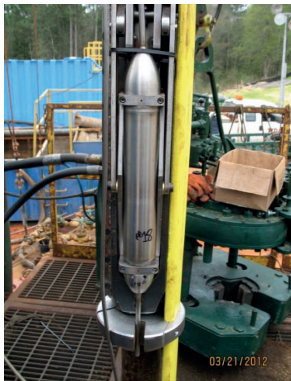
Figure 11. Geophone pod with hydraulic actuated clamp, including flatpack clamped to production tubing.
