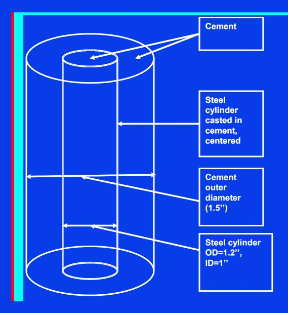
Cement plug with a steel cylinder filled with cement, all castl into one plugs of 32" length
