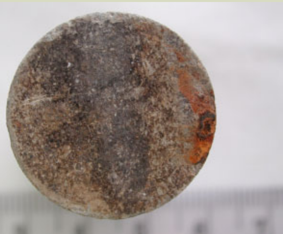
Figure 2.6: Optical view of core from 4560'. An intact contact between casing and cement was preserved during recovery (left image). The surface of the cement plug facing the casing (Right image) had a piece of corroded steel attached to it (orange area). The surface of the cement also had a layer of minute (< 100 mm) reflective crystals (calcium carbonate).
