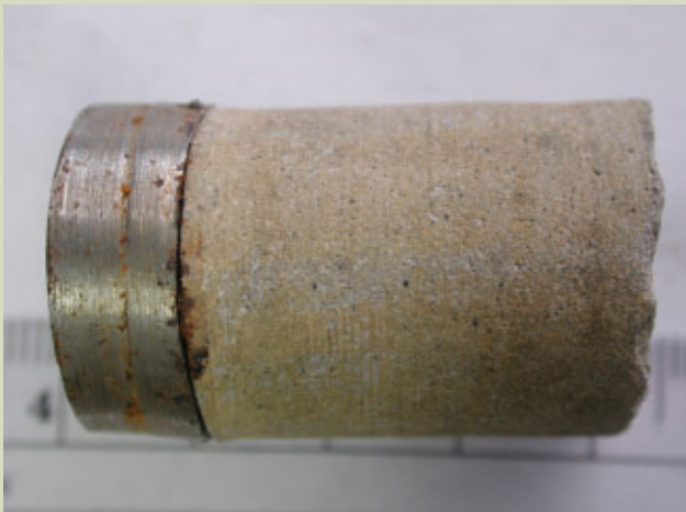
Figure 2.6: Optical view of core from 4560'. An intact contact between casing and cement was preserved during recovery (left image). The surface of the cement plug facing the casing (Right image) had a piece of corroded steel attached to it (orange area). The surface of the cement also had a layer of minute (< 100 mm) reflective crystals (calcium carbonate).
