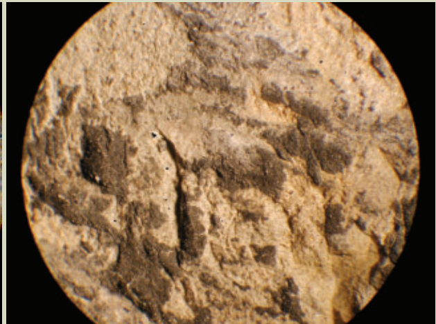
Figure 2.5: Surface of cement core from 4528' depth showing black pieces of shale adhering to the cement surface (view is 5 mm in width).
