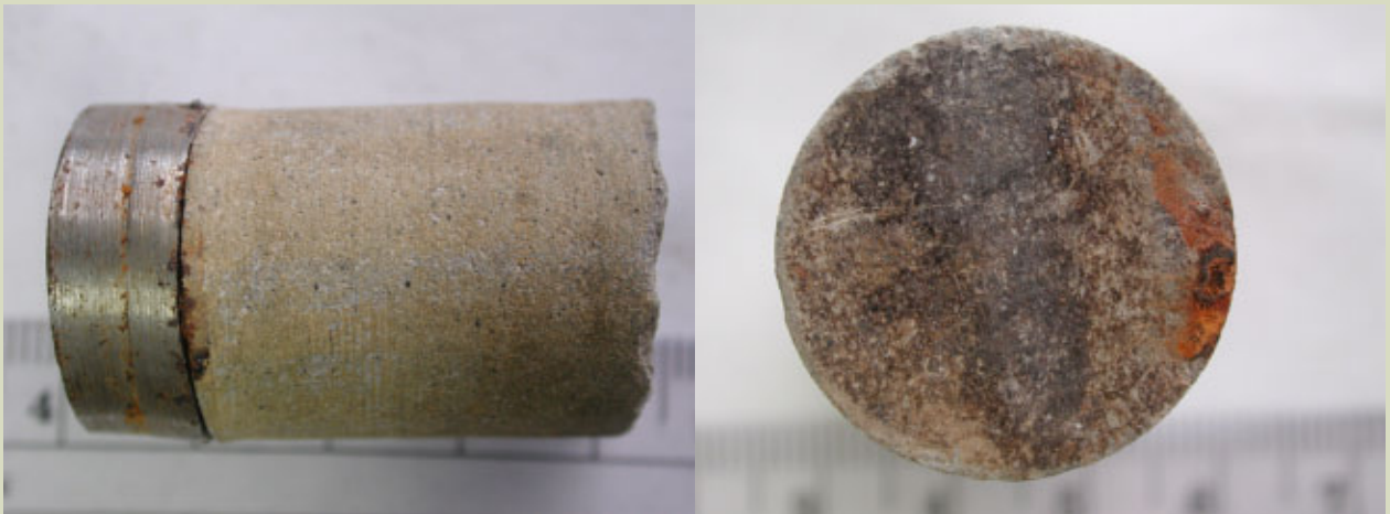
Figure 2.6: Optical view of core from 4560'. An intact contact between casing and cement was preserved during recovery (left image). The surface of the cement plug facing the casing (Right image) had a piece of corroded steel attached to it (orange area). The surface of the cement also had a layer of minute (< 100 nm) reflective crystals (calcium carbonate).
