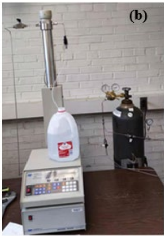
Figure 9. Experimental setup for cement CO 2 degradation. (a) Schematic illustration of the setup. (b) The control station, including the syringe pump, CO 2 tank, pressure gauges, and valves. (c) Pressure vessel and accumulator are placed in an oven under a controlled temperature.
