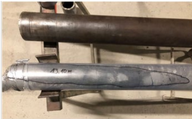
Figure 19. Lateral borehole BCS-A3 (left) last centimeters of sample with OPA/cement interface and parts of the steel casing of the completion.
