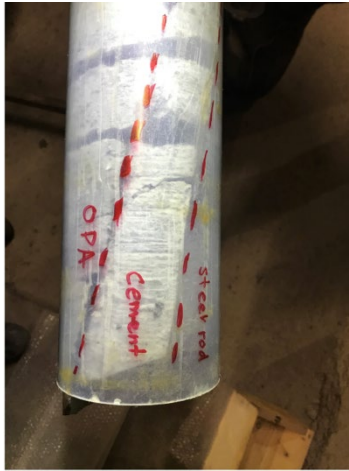
Figure 19. Lateral borehole BCS-A3 (left) last centimeters of sample with OPA/cement interface and parts of the steel casing of the completion.
