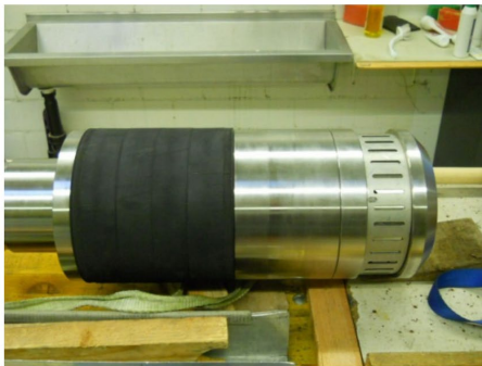
Figure 5. Detail of the injection interval (Interval 1) and grout packer 1.
