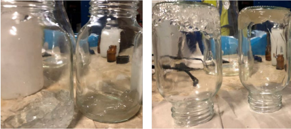
Figure 34 Polymer gel samples: test sample (left in both images) and sample taken at the outlet (right in both images).
