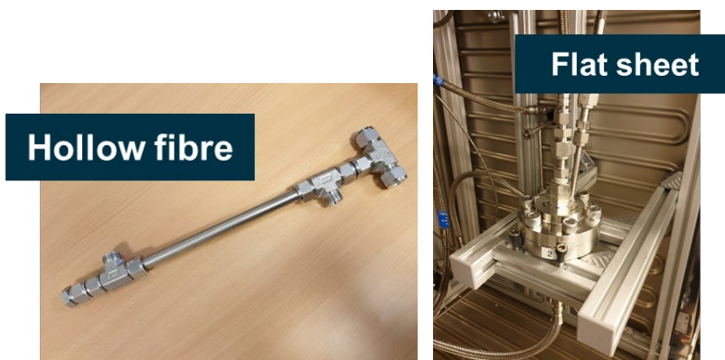
Figure 7. Test configuration of micro-scale membrane modules.
