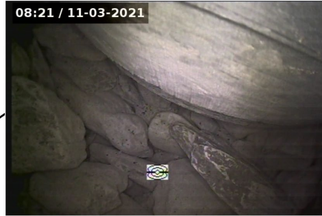
Fig. 7.5m. Broken OPA ring fragments at 7.5 depth at bottom of grout packer. Growing concerns that OPA below grout packer disintegrates and falls down inside inner barrel and is milled away as drilling progresses.
