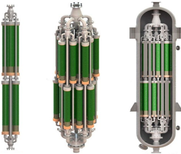
Figure 4. Subsea membrane deployment concept. From left to right: membrane cartridges assembled into a string; the strings are arranged into an insert to a pressure vessel; assembled subsea membrane separator.
