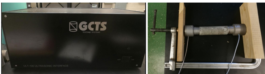
Figure 7. The ultrasonic test interface and setup for testing elastic parameters during cement hardening.
