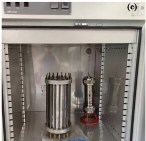
Figure 9. Experimental setup for cement CO 2 degradation. (a) Schematic illustration of the setup. (b) The control station, including the syringe pump, CO 2 tank, pressure gauges, and valves. (c) Pressure vessel and accumulator are placed in an oven under a controlled temperature.
