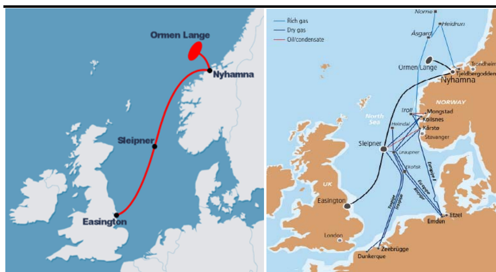
Figure 3.1 Route of the Langeled pipeline route and integration with existing gas transport infrastructure
