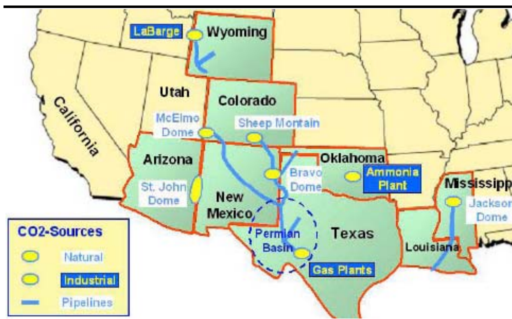
Figure 7.1 Map showing CO 2 sources, transportation pipelines and extent of CO 2 -EOR in the South and South-West United States
