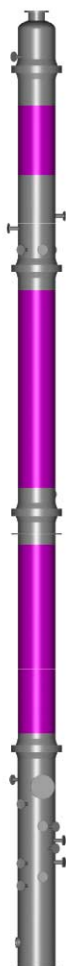
Figure 8: 3D drawing of the absorption tower, pilot unit at K-Lab, Kårstø, Norway. Pink/dark colour illustrates the packing material sections with the water wash at the top.
