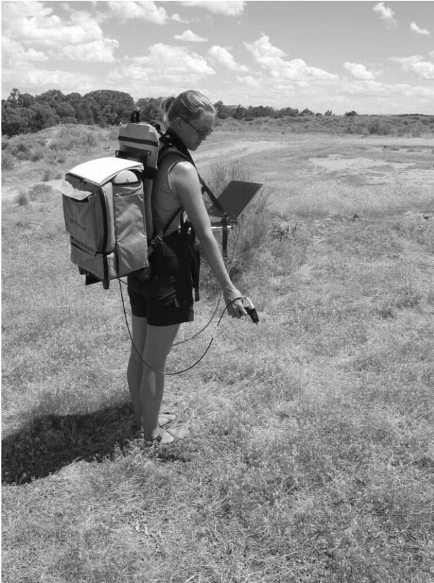
Figure 7: Using the ASD field spectroradiometer to measure reflectance spectra at Rangely in August 2003. The spectrometer is in the backpack. The computer that controls the spectrometer and displays the acquired spectra is in a front pack sling. The pistol grip lens is connected to the spectrometer by a fiber optic cable.
