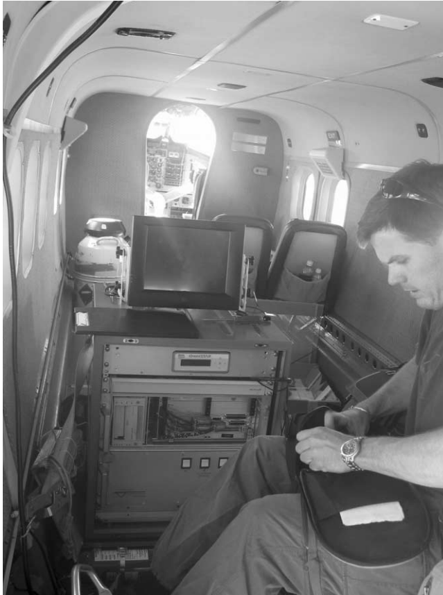
Figure 9: The acquisition contractor’s sensor operator and flight commander. He is shown with the onboard computer system that controls the sensor systems and records the image, and the exact geolocation of each pixel in the image as it is acquired.
