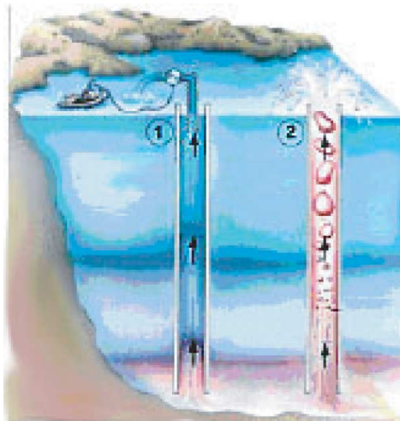
Figure 5: Degassing procedure principle: 1, priming the self-siphon using an electrical pump; 2, autonomous soda fountain ( http://perso.wanadoo.fr/mhalb/nyos/ ).
