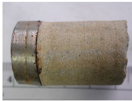
Figure 2.4: Core from 4650' with an intact contact between casing and cement
