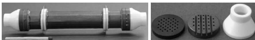
Figure 12. HMR small-scale test module, and a separate choke plate, flow distributor and top hat prior to module assembly.
