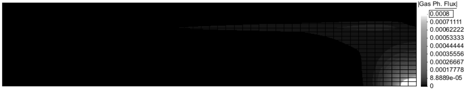
Figure 4. Simulated results of gas phase flux (m/s) after 100 years of CO 2 injection.
