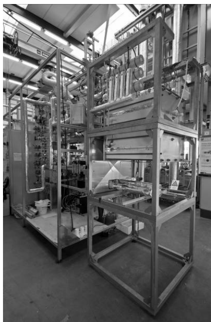
Figure 10. Process Development Unit (PDU) for testing of membrane reactors for CO 2 capture.
