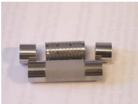
Porous support after polishing and its internal reinforcement tube
