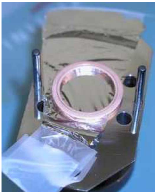
Figure 1: Application of the palladium alloy membrane film onto a flat stainless steel mesh support.
