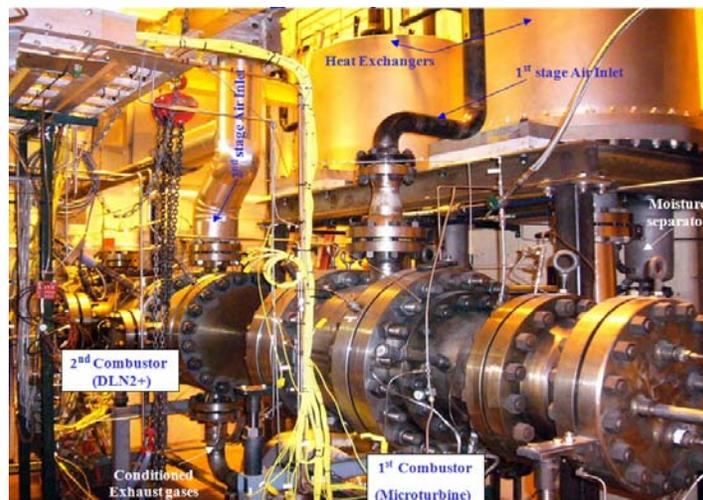
Figure 3 – Test rig as assembled at GE GRC-Niskayuna
